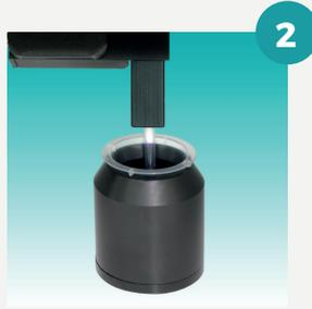
The syringe takes the liquid sample from an irradiated sample beaker.
