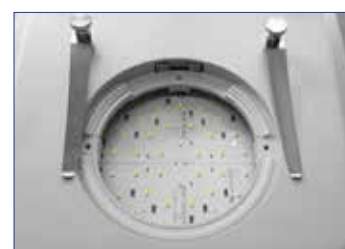
SZ-ST3: 60-Led X-LED™ Transmitted Illuminator
